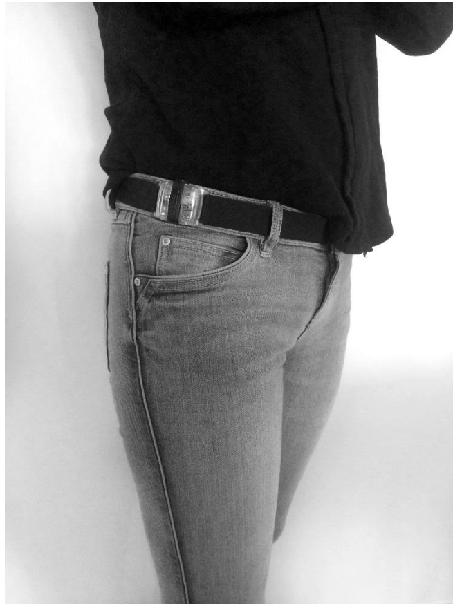
Figure 5. A small and light-weight accelerometer from ActiGraph™ attached on an adjustable elastic band and worn on the right hip.
